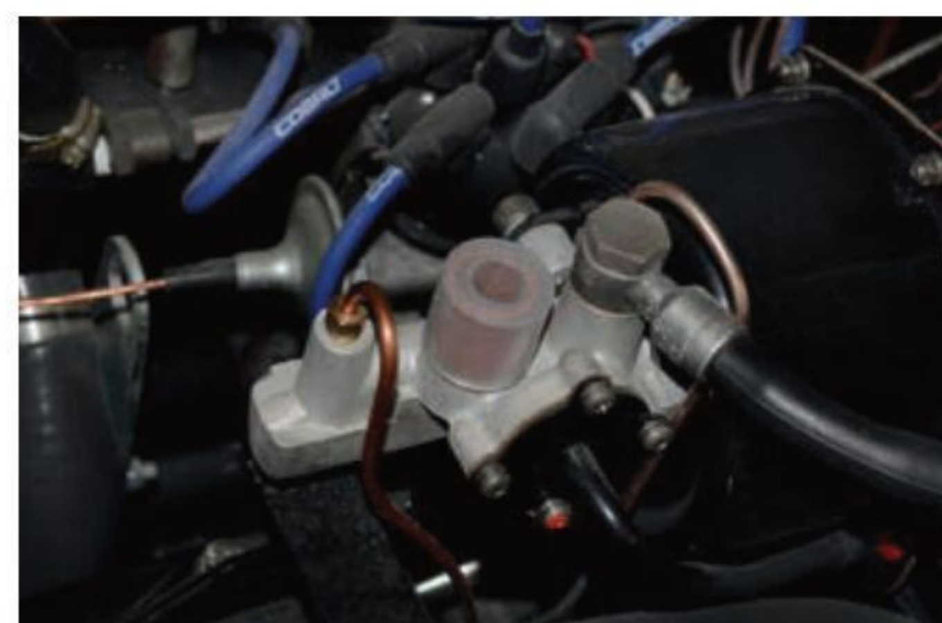
The brake servo and single line brake system are again standard Triumph: the steel-bodied Italia weighs about the same as a TR4, so the same brake system works fine.
