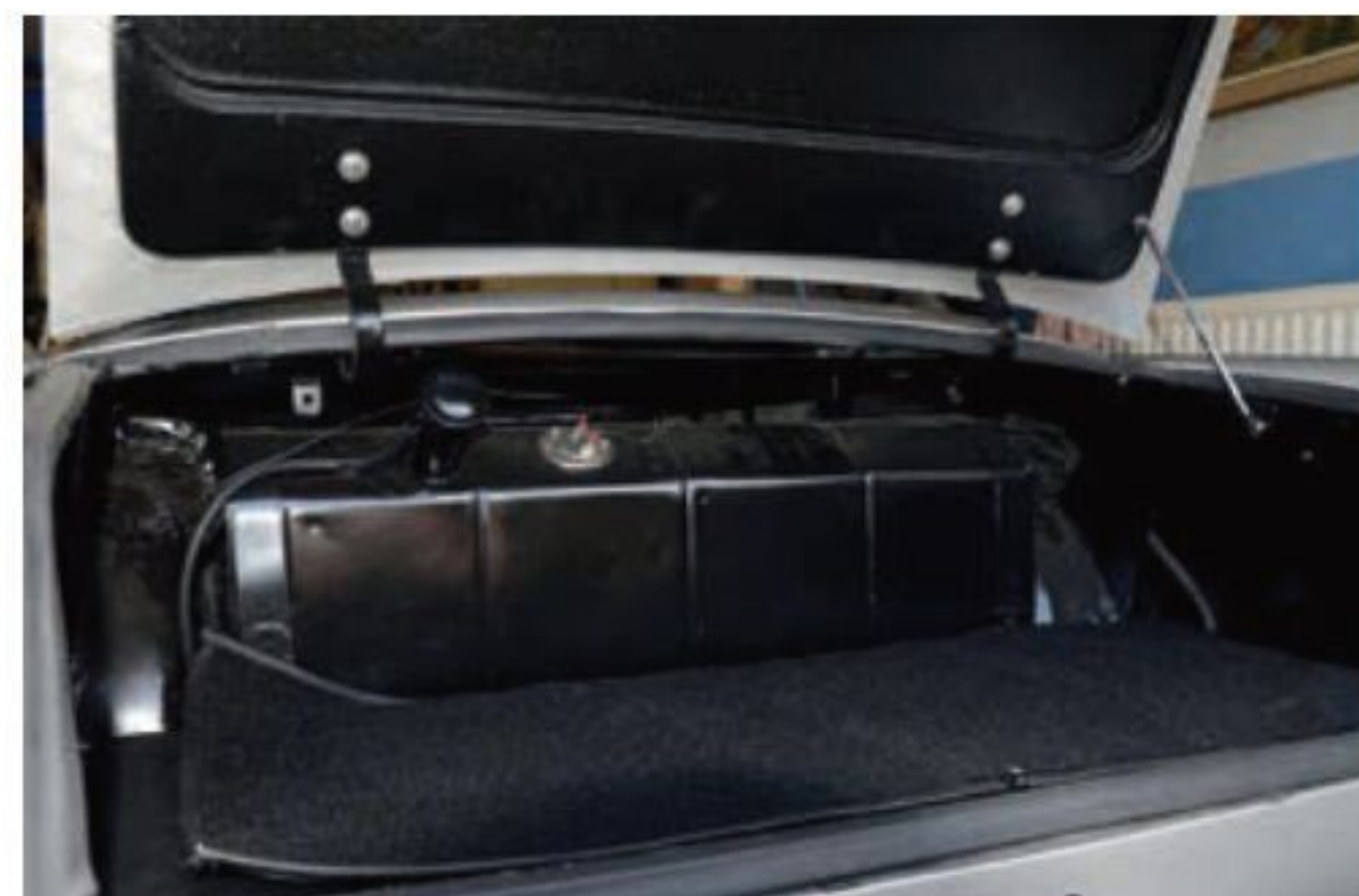
Fuel filler is inside the boot, which keeps it cheap and simple, but also avoids the clutter of external fuel caps or complex hinged fuel cap lids.
