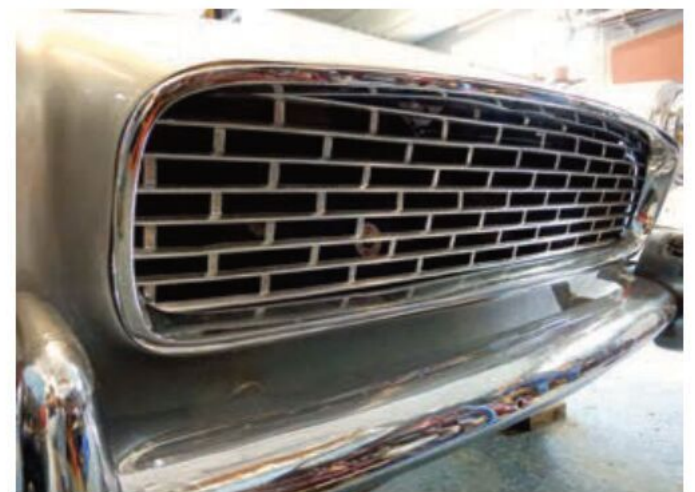
The grille pressing is shared with Maserati. The overriders are a vaguely familiar shape, although the bumper looks custom and fits the body beautifully.
