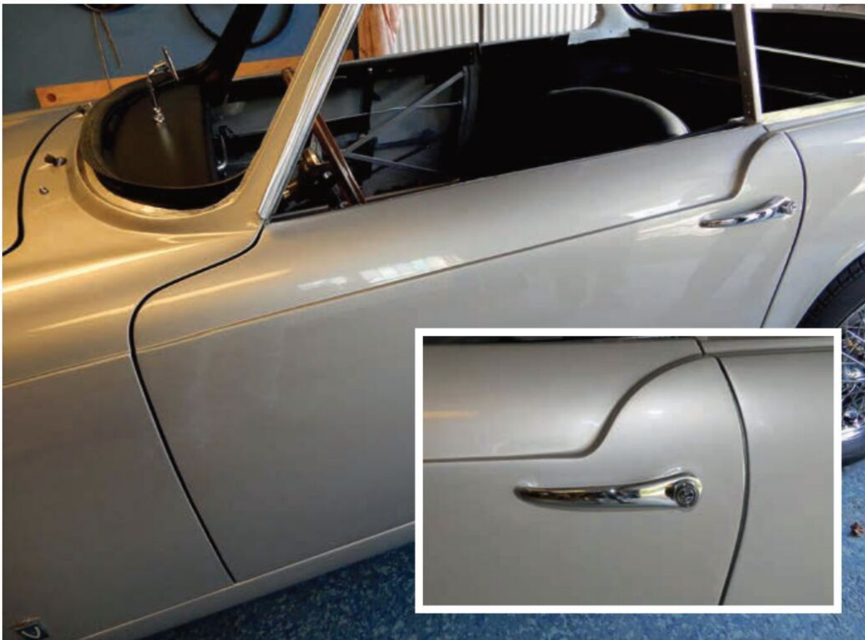
The swage line at the back of the door is very sharp in the Italia, although the TRs lose that definition in the doors. That may well be due to a financial mass-production pressing-tool limitation, but the Italia's doors were handmade so they could be any shape Michelotti wanted.
